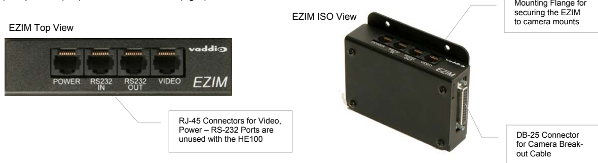
Figure 3: EZCamera Interface Module (EZIM) with four (4) RJ-45 connectors for POWER, RS-232 IN & OUT and VIDEO (HD or SD with IR), Top View (left) and Isometric View (right)
