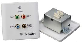
The Intelix AVO-V3AD-WP110-EU wallplate balun transmits one component video and one digital audio signal over standard unshielded twisted pair cabling, such as Cat 5 or Cat 6. Used in pairs or with a compatible Intelix balun, the AVO-V3AD-WP110-EU transmits signals up to 500 feet and is ideal for corporate A/V, churches, schools, auditoriums, and almost any other situation involving audio/video distribution.
