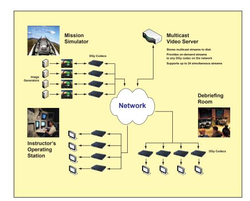
RGB Spectrum's Multicast Video Server (MVS) simultaneously records, stores, and multicast streams from 6 to 24 channels, offering the powerful capability to record and store multiple channels while viewing the same imagery at multiple locations.
