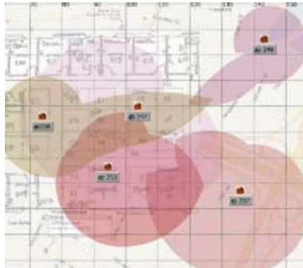
Coverage gap detection tool in Firetide WLAN Controller
