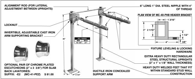
NOTE: Foot supports should be securely anchored to floor with  $\frac{1}{2}$ " bolts and anchors by others
