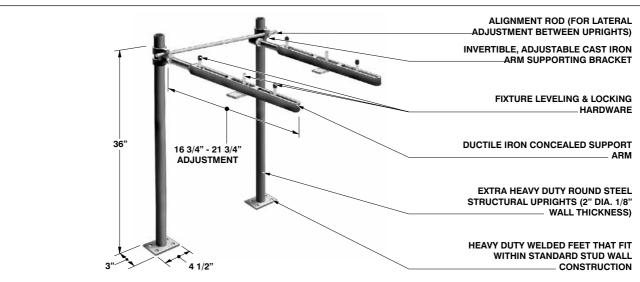
NOTE: Foot supports should be securely anchored to floor with ½" bolts and anchors by others
