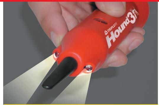
The New Hound 3 Probe features 2 Bright, White LED Headlights that will help light your way in dark areas or reduce fluorescent light noise by allowing you to turn off overhead lighting.
