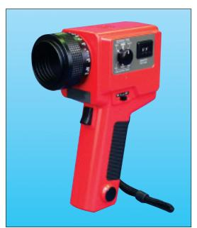
DHS55 – For Liquid Metals - is designed for accurate temperature measurement of liquid metals in iron and steel foundries. The thermometer automatically compensates for ambient temperature changes, and provides a fast response time (0.8 seconds) and reliable reading in the extended range of 1830° to 3270°F (1000° to 1800°C). Short wavelength operation (0.55 $\mu$ m) minimizes errors due to emissivity/atmospheric absorption.
