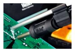
Weller® FE soldering irons feature a smoke absorption tube integrated into the handle. It can be placed over the joint when soldering, but can be retracted when access to the joint is a problem. It can also be removed for cleaning. The irons are temperature controlled, ergonomic, and allow precise handling. These
