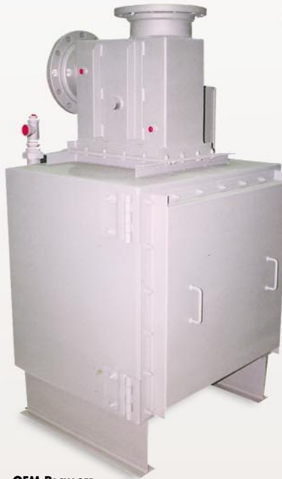
OEM PACKAGER, Model HRSR-112C26.5ALS Recovering Btu from (1) 75 kW Micro Turbine Generator, natural gas engine. Reducing each 500°F @ 1,198 SCFM to 213°F; Raising 35 GPM hot water from 160°F to 181°F.
