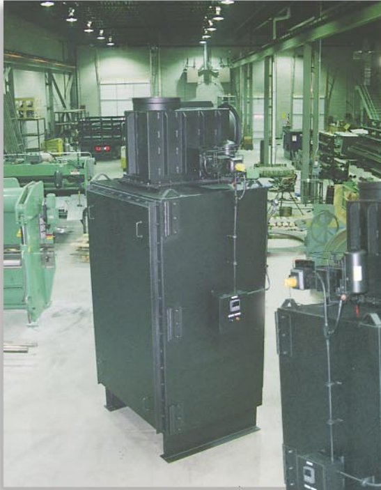
HOSPITAL, Ontario (2) Model HRSR-336B28CSS Recovering Btu from (2) Cummins Wartsila CW180, natural gas engines. Reducing each 968°F @ 3,666 SCFM to 339°F. Raising 175 GPM hot water from 195°F to 229°F.
