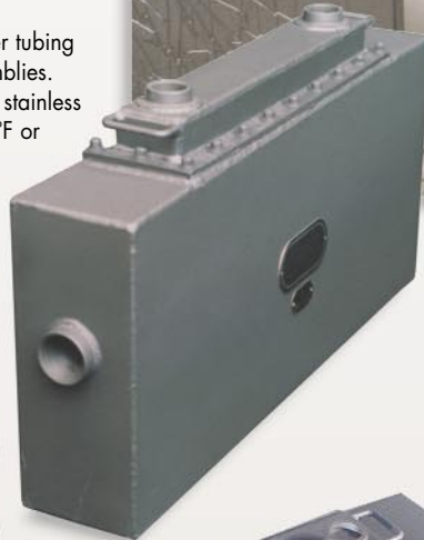
MOBILE TRAILER , Venice, California Model UTR-630218CSS. Recovering Btu from a 33kW natural gas engine. Reducing 1,282°F @ 76 SCFM to 319°F; Raising 27 GPM 50% ethylene glycol from 190°F to 198°F
