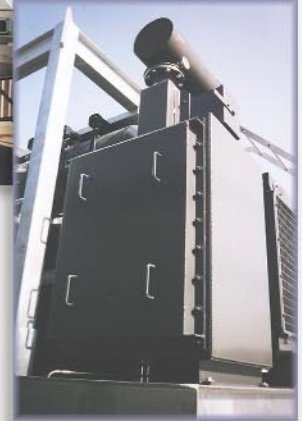
(2) MOBILE TRAILERS, (2) Model HRSR-216826SSS Recovering Btu from a diesel fueled N14 Cummins engine Reducing each 865°F @ 1,188 SCFM to 465°F. Raising 70 GPM 50% Ethylene Glycol from 70°F to 90°F.
