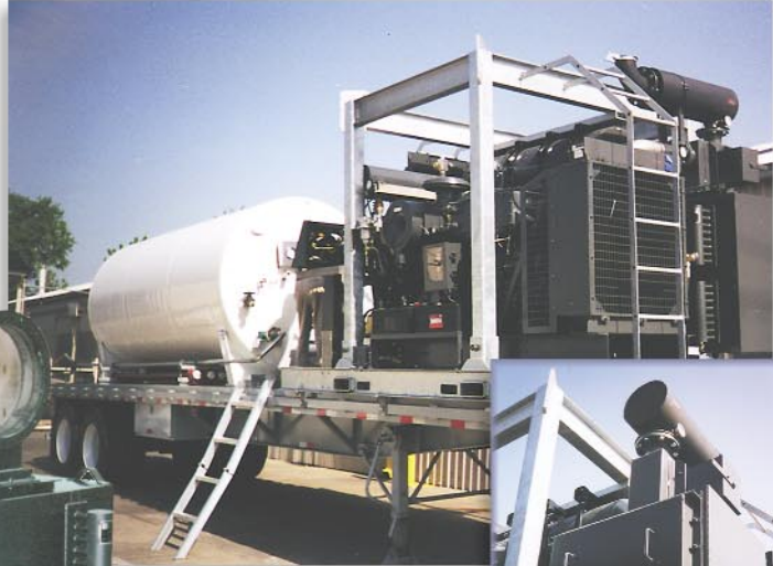
(2) MOBILE TRAILERS, (2) Model HRSR-216826SSS Recovering Btu from a diesel fueled N14 Cummins engine Reducing each 865°F @ 1,188 SCFM to 465°F. Raising 70 GPM 50% Ethylene Glycol from 70°F to 90°F.
