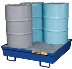
Steel Pallets constructed of 11 gauge hot rolled steel and strengthened with formed edging feature generous sump capacities and are 100% tested leaktight. Galvanized steel bar grating keeps drums out of overflow and remove for easy cleaning. Large forklift pockets (8-3/8"w x 3-7/8"h, 213mm x 98mm) in front and back make relocation easy. Users choice of two finishes: tough
