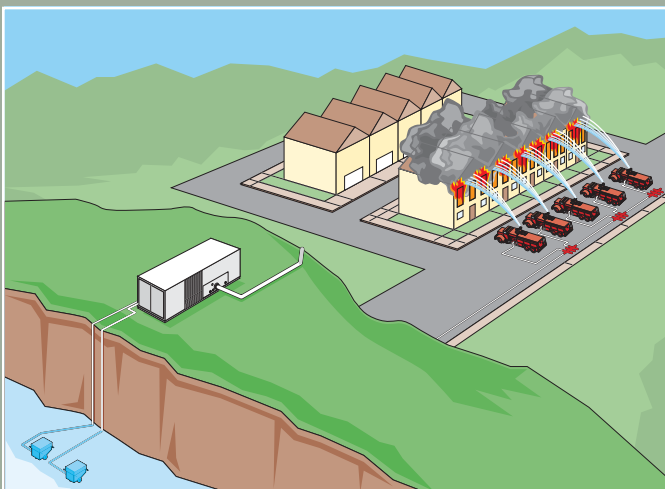
Pumping to Multiple Devices and Apparatus
