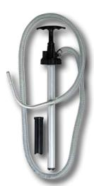
Optional piston style hand pump with aluminum no-drip tip allows users to quickly and neatly dispense industrial fluids into hard-toreach areas without having to hold the drum. The five foot (1.5 meter) flexible hose has a metal reinforcing wire imbedded within the hose so it doesn't contact the fluid.
