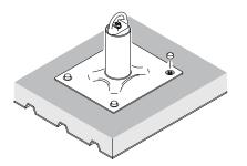
**Step 3**Tighten each bolt and install protective cap
