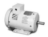
**Features:** Class F insulated motor with 1.15 service factor or higher that operates within class "B" temperature limits at rated horsepower. Moisture resistant insulation system. Top mounted F3 conduit box. Sealed ball bearings with moisture-resistant grease. C-Face motor windings are epoxy encapsulated for added moisture protection.
