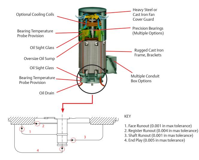
Emerson is proud to offer products that meet the stringent requirements for motors used with API 610 pumps in Petrochemical Industries. The API 610 option is available on 400 frame sizes and larger on both open and enclosed motor types.
