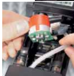
Measurement cells can be easily changed by user without test gas
