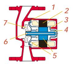
stainless steel stator can isolates the stator from system fluid and maintains precision bearing alignment for longer bearing life
