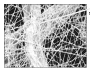
Nanofiber filter media combines both large and small fibers to trap more particle sizes without restricting airflow.
