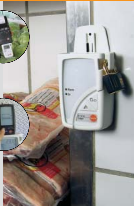
Long-term temperature logging in an intermediate store with testo 177-T1 (without display)
