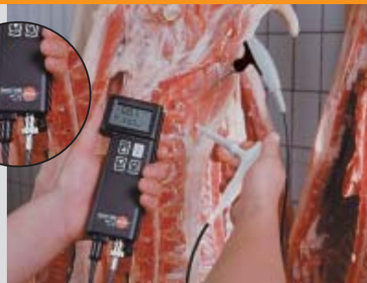
Checks pH value and penetration temperature in meat prior to further processing
