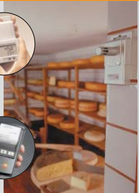
Monitors humidity and temperature in storage rooms
