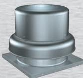
The spun aluminum downblast centrifugal roof exhaust fan models G and GB (direct or belt drive) are an economical means of exhausting air. They utilize a backward-inclined wheel and are available in 45 different sizes. Capacities range from 50 to 44,700 cfm and up to 3.25 in. wg of static pressure.
