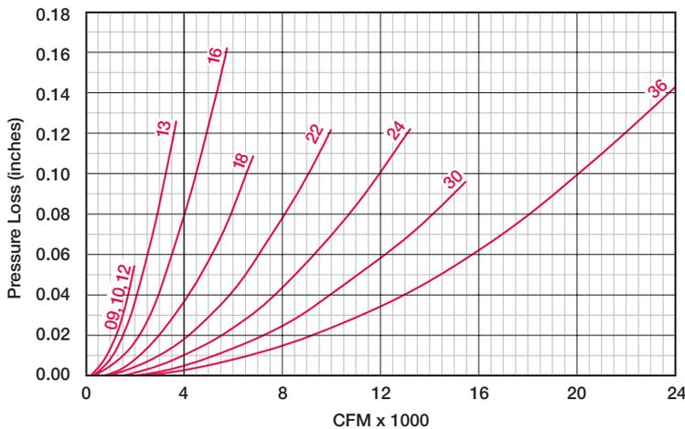
TCBRS fan selections can be made using the TCB inline performance data (pgs. 12 to 31) along with the following system effect curves. The pressure loss determined to the left must be added to the external system static pressure to assure accurate selections. Greenheck's Computer Aided Product Selection (CAPS) software will add these system effects automatically.
