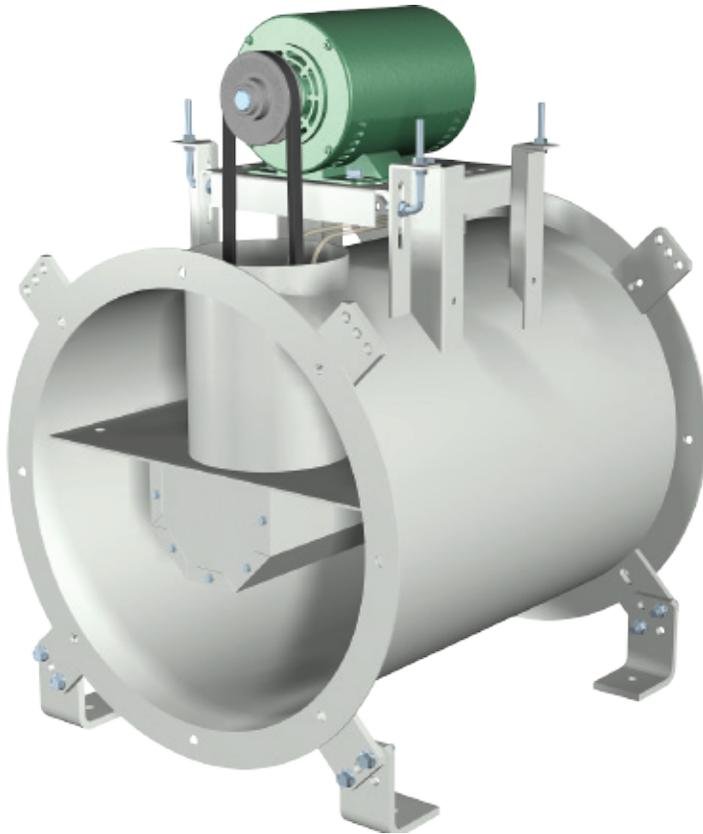
The Model TCB inline fan is the ideal choice for ducted systems. Greenheck's standard fan can be mounted in any position from horizontal to vertical, allowing installation in the smallest possible space at the lowest installation cost. The centrifugal wheels used in this design provide higher efficiencies and lower sound levels than propeller type inline fans when used in medium pressure ducted systems. TCB fans are available in either painted steel or aluminum construction.
