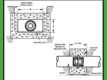
Terra-Gard Unit Joining Method
