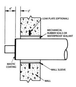
It is recommended that all building or manhole entries be sleeved and that the annular space between the jacket and sleeve be sealed with either a mechanical rubber seal or a waterproof sealant. Wall sleeve and mechanical rubber seals are available from PERMA-PIPE. All terminal units must have ends sealed against moisture intrusion. PERMA-PIPE factory seals all terminal ends.
