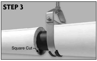
Square cut adjoining insulation and butt the insulation ends to each other.
