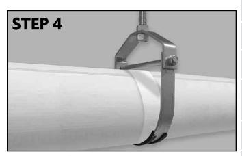
Caulk joints and finish taping.
