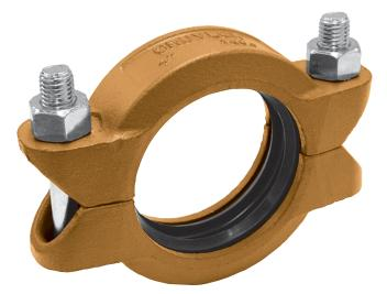
The Gruvlok Fig. 7004 Coupling with EG® Gasket uses the specially designed "End Guard" gasket with "EG" grooved pipe. The "EG" gasket has a center rib which extends between the pipes to provide for pipe end protection which makes it ideally suited for internally lined or coated pipe applications.
