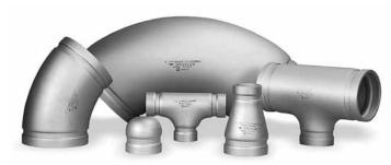
Gruvlok Aseries Stainless Steel Fittings are full flow design with ends grooved to Gruvlok specifications. The 🗲 Series standard material is formed from Type 304 Stainless Steel. The Eseries Fittings are annealed after forming and grooving to provide increased corrosion resistance. Gruvlok 🗸 Series Stainless Steel 45° and 90° elbows and tees have compact centerto-end dimensions which make installation quick and easy with the Gruvlok Figure 7400SS Coupling, or other Gruvlok products.
