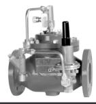
The model 108FPS is used to prevent the fire pump from outdrawing the available supply. In so doing, it protects the pump suction supply from damage associated with a pressure that is too low or backflow and assures adequate supply pressure to the fire system components.
