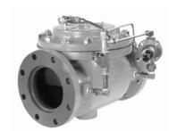
The Apollo Series A115 Solenoid Control Valve is designed to provide on/off or open/close control of fluids in response to an electrical signal. The valve consists of the basic Apollo model A65 with solenoid-operated pilot. With the appropriate solenoid, the valve may be normally closed (energize to open) or normally open (energize to close).
