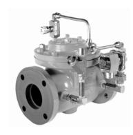
The Apollo A110 Series Differential Control Valve is designed to accurately control the pressure difference between any two points. In some systems this means the valve remains closed until pressure differential commands its opening. It is a pilot operated, modulating type valve which controls pressure accurately and consistently at the desired setting.
