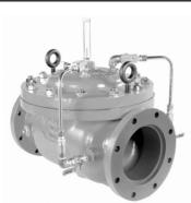
The Apollo Series A94 Check Valve is a simple on-off valve that opens to allow forward flow when inlet pressure exceeds outlet and closes tightly to prevent backflow when outlet pressure exceeds inlet pressure.
