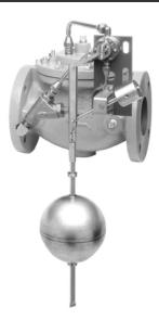
The Apollo Series A800 Float Control Valves are designed to maintain a desired level in a tank or reservoir by opening for filling the tank when fluid is below the high level point and closing tightly when the desired level is reached.
