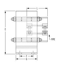
Pipe Size L **Maximum** (in) (in) Movement 1" to 6" 6 6 8" to 16" 8 8 18" to 24" 10 10
