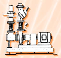
The valve stem with its grooved rings and positioning sleeve indicates the throttled position of the valve. The quarter turn graduations on the sleeve, with the scribed line on the stem, provide for approximate flow measurement.
