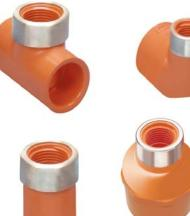
Spears<sup>®</sup> patented special reinforced (SR) plastic female thread design is one of the most significant advancements in the use of CPVC fire sprinkler system threaded fittings. Not just an added ring, this unique precompression design compensates for expansion forces generated from tapered pipe thread joint makeup. Radial stress is no longer a problem in normal installations and easily managed in severe over-tightening situations.
