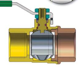
**Full port brass valves** The spindle, assembled from inside, is blow-out proof. The high quality PTFE is a guarantee of long endurance and excellent seal. The body and ball are made of CW617N brass.
