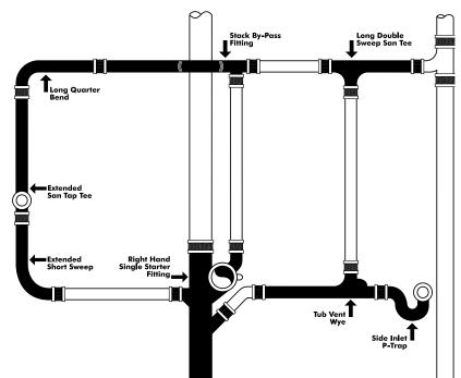
The **by-pass fitting** permits in-line piping to reduce width of the chase, and individual venting of the lavatories.
