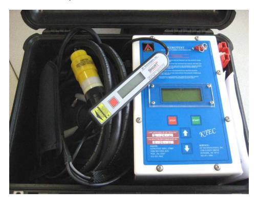
KTEC Electrofusion Control Box Fusion capabilities: (KTEC weight: 21 pounds)
