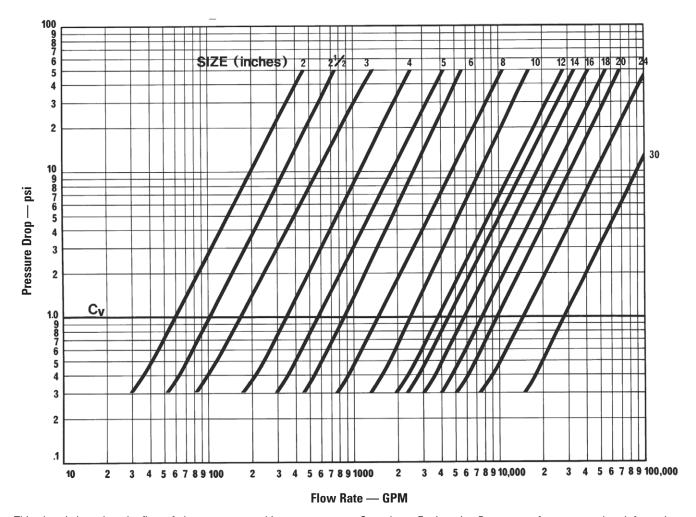
This chart is based on the flow of clean water at ambient temperature. Consult our Engineering Department for pressure drop information for steam, gases or viscous fluids.
