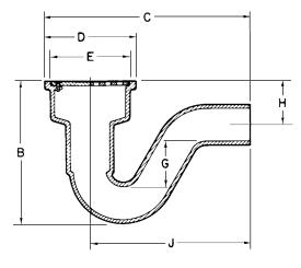
732 Cast Iron Body with Integral P-Trap (Omaha Code) Spigot Outlet only Shipped with Perforated Cast Iron Strainer, Not Threaded for Back Water Valve Fits SV Ty-Seal® gasket or may be joined with Tyler No-Hub Coupling
