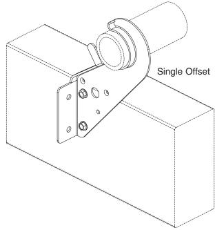
Install using a rechargeable electric drill fitted with a 5/16" socket attachment with the special hex head self-tapping screws provided. Install screws until they bottom out. Pipe can be "snapped" into hanger before or after installation of the screws to the mounting surface. "Thumb tab" may be bent up to provide additional protection to the pipe, but is not required for performance of the hanger / restrainer function.
