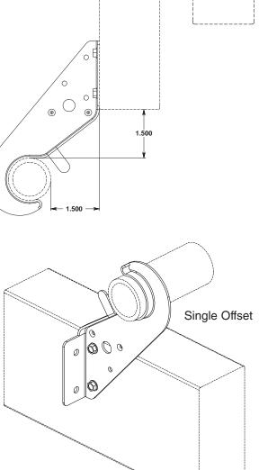
Install using a rechargeable electric drill fitted with a 5/16" socket attachment with the special hex head self-tapping screws provided. Install screws until they bottom out. Pipe can be "snapped" into hanger before or after installation of the screws to the mounting surface. "Thumb tab" may be bent up to provide additional protection to the pipe, but is not required for performance of the hanger / restrainer function.
