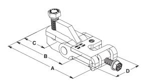
**Installation** — The Fig. 981 is the "braced pipe" attachment component of a lateral or longitudinal brace assembly. It is intended to be combined with the pipe hanger, all-thread rod, "bracing pipe" and TOLCO transitional and structural attachment component(s) to form a complete bracing assembly. NFPA 13 and or OSHPD guidelines should be followed.
