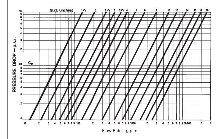
Above based on the flow of clean water through .033: - ¼" perforated metal screens. Consult our Engineering Department for pressure drop information on steam, gases or viscous fluids. See Theoretical Pressure Drop Curves for Screen Clogging In the Technical Data Section for multiplying factors for clogged screens.
