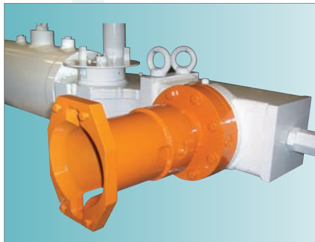
ISO 13628-8 Class 4 ROV receptacle for rotary torque tool operation of the actuator mechanical over-ride.
