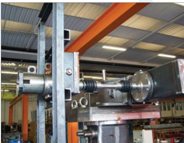
Stainless steel drive extensions for remote location of ISO 13628-8 rotary torque tool receptacle.
