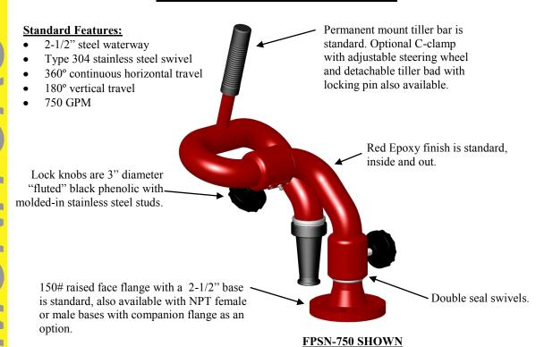
**Potter Roemer / Fire Pro**® offers model in this configuration feature a 180-degree vertical travel that is ideal for tank cleaning and any other wash down applications. Like all monitors from Fire Pro® heavy-duty construction and red epoxy finish stand up to the rigorous uses found in municipal and industrial environments.
