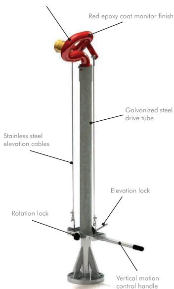
**Freestanding monitors** have an "inner" waterway with an outer drive tube for horizontal movement at the base, along with vertical motion handle control with stainless steel cable attached to the monitor for vertical option.
