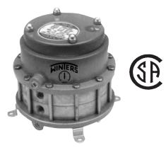
Ranges from 0-1.5" WC to 0-150" WC Rugged NEMA 4X and 12 housing standard CSA Certified Class I, Div. I, Gr. C and D available Up to four SPDT contacts Various wetted materials available
