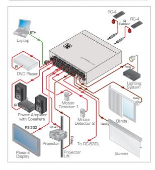
The SL-12 is a highly versatile controller that acts as an all-in-one extended remote control for control of A/V equipment. It streamlines operations and simplifies control by integrating audio, video, and computer-video sources into a centralized system
