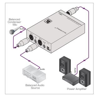
The 102xl is a high-performance 2-channel mono audio mixer for line level and mic level balanced audio signals. The unit mixes two mono inputs and produces a mixed audio output signal.
