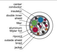
Kramer's BC-3X2T7S is a high-resolution multi-conductor containing 3 mini coaxes, 2 shielded pairs, and 7 single strands. It is the most common type of cable used for construction of 15-pin HD (VGA/UXGA) cables.
