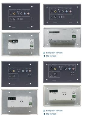
The WP-27 and WP-28 are a twisted pair transmitter and receiver for composite video, s-Video, or component video and unbalanced stereo or S/PDIF audio signals. The WP-27 converts a single audio and video input into a twisted pair signal and the WP-28 converts the twisted pair signal back into the original audio and video formats.
