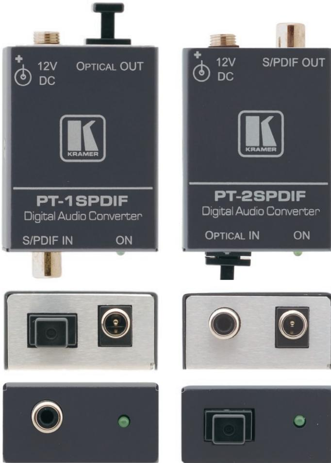
The **PT-1SPDIF** and **PT-2SPDIF** are format converters for S/PDIF and TOSLINK® digital audio signals. The **PT-1SPDIF** converts an S/PDIF signal to a TOSLINK® optical signal. The **PT-2SPDIF** converts a TOSLINK® optical signal to an S/PDIF signal.
